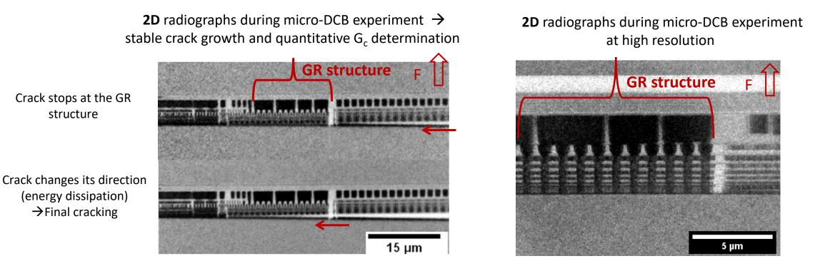
FOV: 65  $\mu$ m or 16  $\mu$ m; Resolution 100 nm or 50 nm
