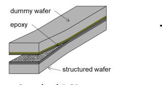
Standard DCB test: (ex-situ) fracture mechanics  $\rightarrow$  G<sub>c</sub>
