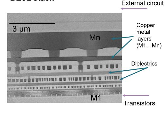
Example: Cu/ dielectric on-chip interconnect stack of advanced ICs (14 nm CMOS technology node)
