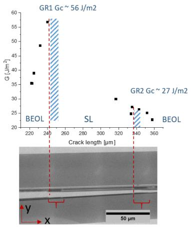
**3D** data during or after micro-DCB experiment  $\rightarrow$  detailed crack path investigation at selected ROI 3D reconstructed data at different loading steps
