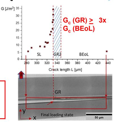
Calculated G values at several loading steps (and respective crack lengths) and stitched image of the final loading stage in the BEoL region
