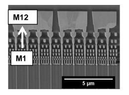
SEM image of a cross-section with GR structure of a microprocessor chip with 12 copper layers (M1 to M12)
