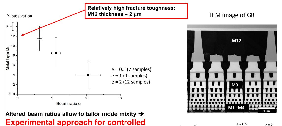
**Experimental approach for controlled microcrack steering**; preferably to regions of high  $h_1 - beam height 1 (Dummy)$   $h_2 - beam height 2 (Chip)$  e = 0.5 e = 2 $\begin{pmatrix} \bullet & h_1 \\ h_2 \\ h_2$
