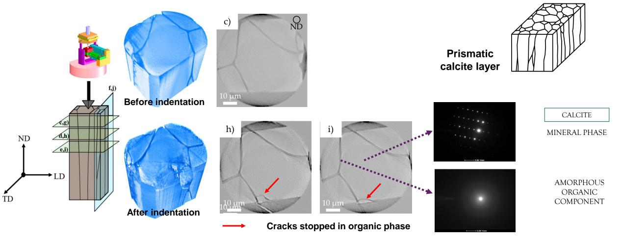
Cracks formed by indentation propagate in the calcite prism and are stopped in the organic phase
