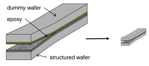
Standard DCB test: (ex-situ) fracture mechanics  $\rightarrow$  G<sub>c</sub> Miniaturized DCB: <u>in-situ</u> 3D crack evolution using X-ray microscopy
