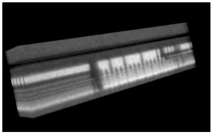
3D data during or after micro-DCB experiment → detailed crack path investigation
