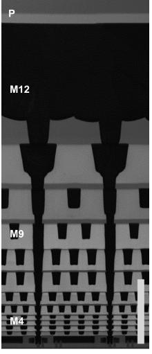
Cu structures > 1  $\mu$ m: Increase of fracture toughness / G<sub>c</sub> !
