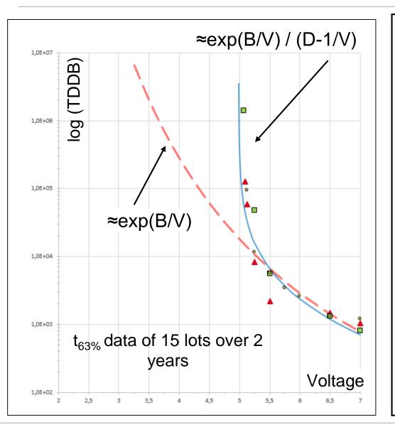
✤ Applying the 1<sup>st</sup> tube equation t<sub>I</sub> x f x (G<sub>n</sub> –G<sub>th</sub>) = C<sub>t</sub> in combination with FN-equation results in
