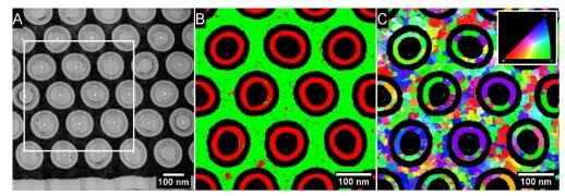
Phase and orientation analysis of 3D-NAND devices
